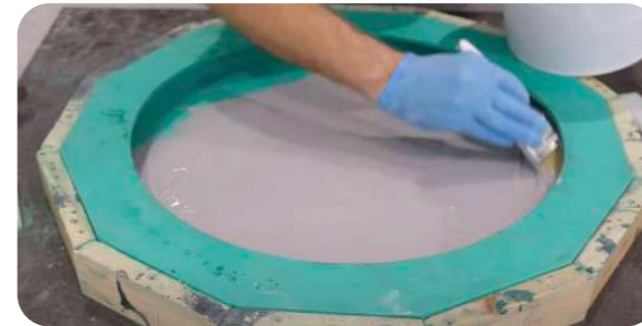
Step Five Brush 1-2mm layer into mould for best results.
